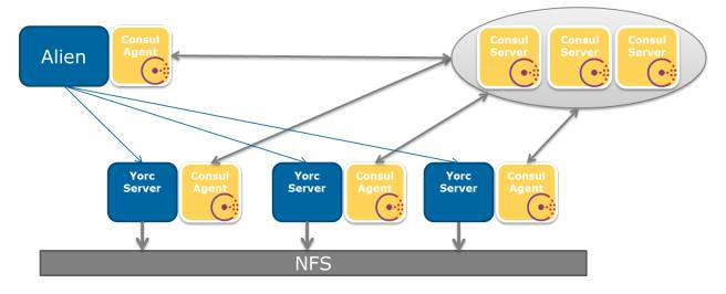
The bellow figure illustrates how a typical Yorc setup for enabling High Availability looks like.
